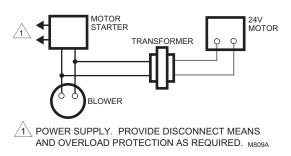
Fig. 10. Wiring connections for Series 81 Motors controlling two-position pre-heat coil valves.
