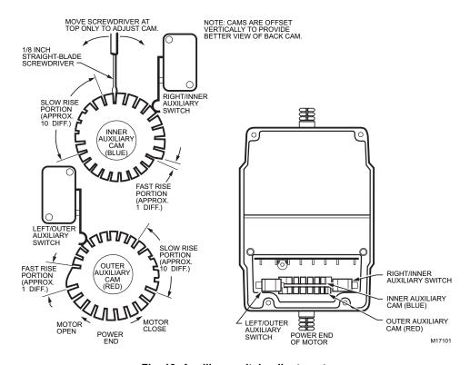
Fig. 13. Auxiliary switch adjustments.
