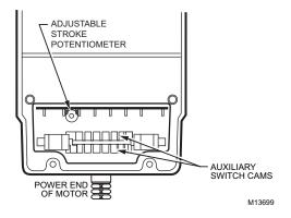
Fig. 11. Stroke adjustments.
