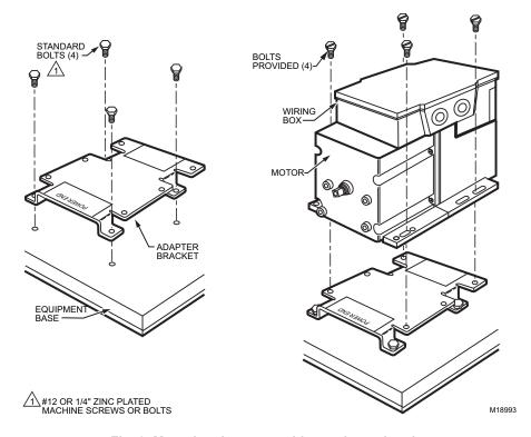
Fig. 3. Mounting the motor with an adapter bracket.
