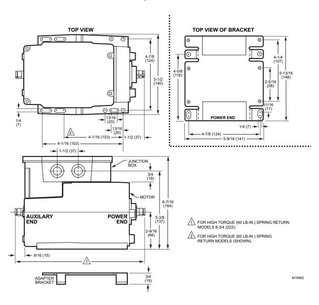
Fig. 2. Series 41 and Series 81 Modutrol IV Motor mounting dimensions in inches (mm).
