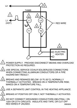
Fig. 3. Typical hookup for T498B Thermostat.
