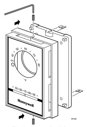
Fig. 4. Locking cover installation.
