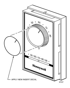
Fig. 6. Thermostat recalibration.
