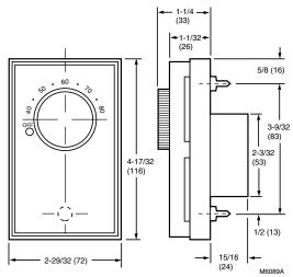
Fig. 1. Nominal dimensions in in. (mm).
