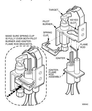
**IMPORTANT:** Make sure the assembly is oriented in the proper direction for installation into the pilot burner.
