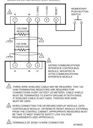
Fig. 5. Wiring the Keyboard Display Module.
