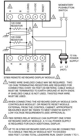
2 TO 2, 3 TO 3 AND PROVIDE 13 Vdc POWER SUPPLY FOR EACH S7800 DISPLAY. TERMINALS OF 203541 5-WIRE CONNECTOR. M5006G
