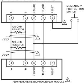
THREE WIRE SHIELDED CABLE MAY BE REQUIRED. TWO 120 OHM TERMINATING RESISTORS ARE REQUIRED FOR CONNECTIONS OVER 100 FEET. CABLE SHIELD MUST BE TERMINATED TO EARTH GROUND AT BOTH ENDS. IF SHIELDED CABLE IS NOT USED, TWISTED PAIR WIRE MUST BE USED.
