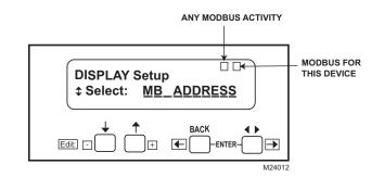
Fig. 31. ModBus activity as viewed on Setup screen.
