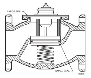
Fig. 2. Placement of valve and bonnet seals in the four-inch valve.
