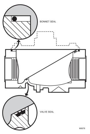
Fig. 1. Placement of valve and bonnet seals.
