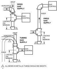
CAUTION: SHUT OFF THE MAIN GAS SUPPLY BEFORE REMOVING END CAP TO PREVENT GAS FROM FILLING THE WORK AREA. TEST FOR GAS LEAKAGE WHEN INSTALLATION IS COMPLETE. M3077
