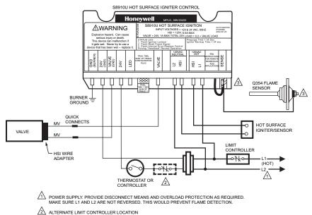
SENSE TERMINAL AND Q354 FLAME SENSOR ON D MODELS ONLY.
