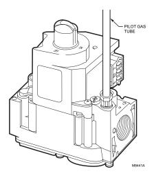
Fig. 6. Remove pilot gas seal (plug) and install pilot gas tube for intermittent pilot application on VR8345.
