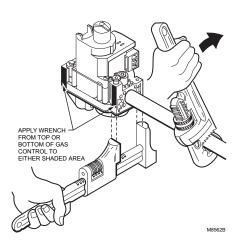
Fig. 4. Proper use of wrench on gas control.
