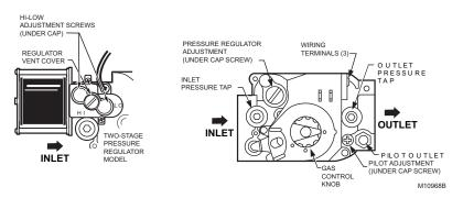
Fig. 3. Top view of gas control.
