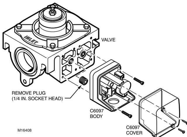
**Fig. 6. Connecting C6097 Pressure Switch to Valve.**
