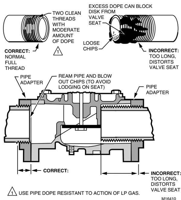
Fig. 1. Preparing pipes.
