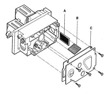
A Screen B Pilot filter \* C Gasket
