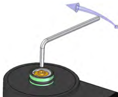
Figure 22: Adjusting flow rate.
