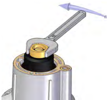
Figure 24: Adjusting flow rate.
